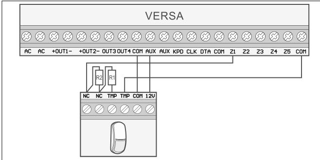
Fig. 25. Example of connecting an NC detector in Double EOL (2EOL) configuration (NO detector connect in the same way).
