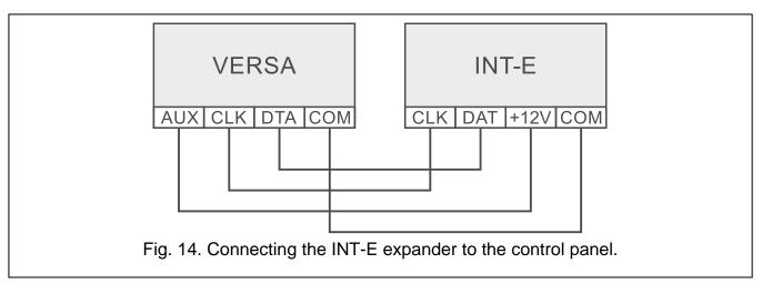
Up to three INT-E / CA-64 E / CA-64 EPS expanders can be connected to the control panel. This enables expansion of the system by adding up to 24 programmable wired zones. Using the expander DIP-switches:
