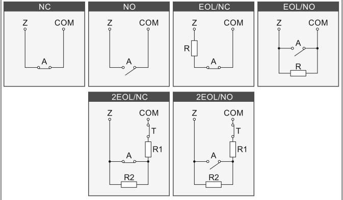
Fig. 21. The ways to connect detectors to zones. The detector outputs are designated with letters: A - alarm, T – tamper. R=R1+R2.
