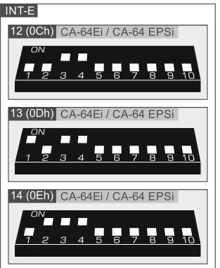
Fig. 15. Setting the DIP-switches in expanders to be identified as CA-64 Ei / CA-64 EPSi.
