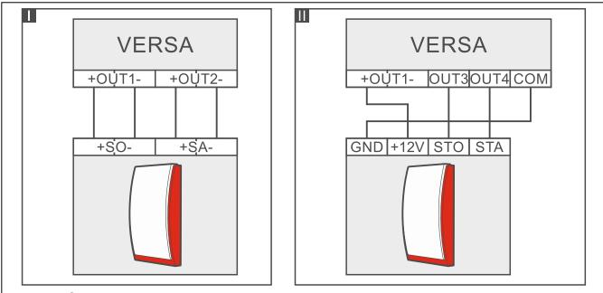
Fig. 26. Connecting sirens to the control panel outputs. I – siren without own power supply. II - siren with own power supply.
