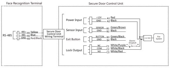
Figure 4-5 Wire Secure Door Control Unit
