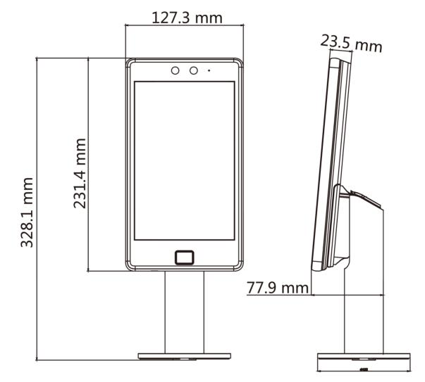
Figure D-2 Dimension with Bracket
