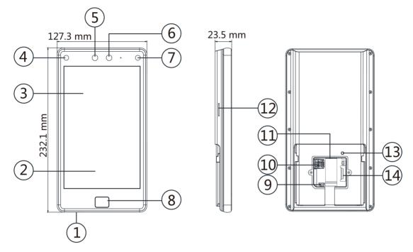
Figure 2-1 Face Recognition Terminal Diagram
