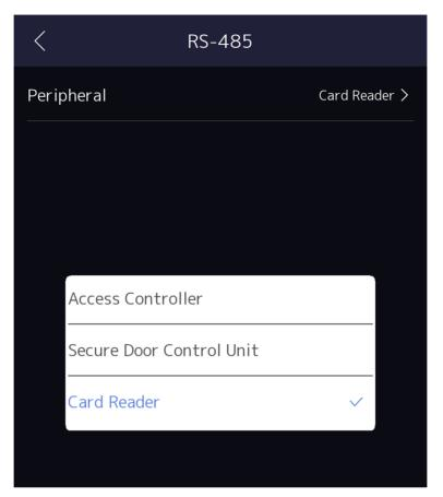
Figure 7-7 Set RS-485 Parameters
