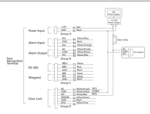
Figure 4-8 Device Wiring
