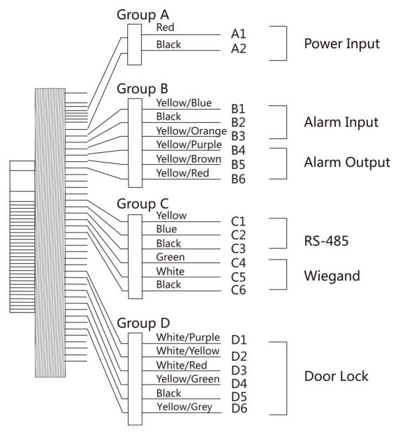
Figure 4-1 Terminal Diagram
