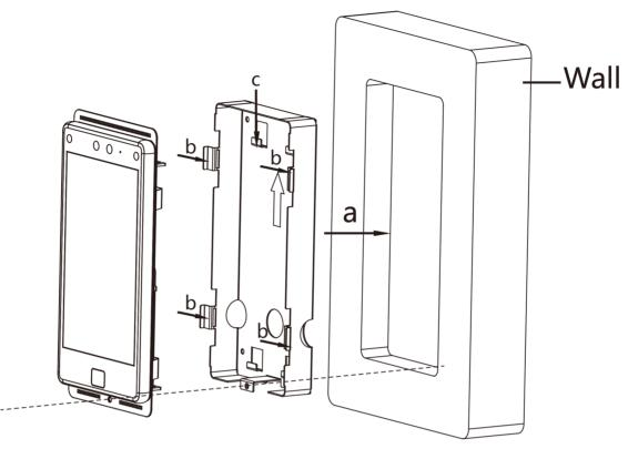
Figure 3-3 Secure the Combination and the Gang Box
