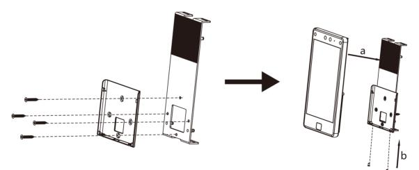
Figure 3-1 Secure the Device on the mounting plate
