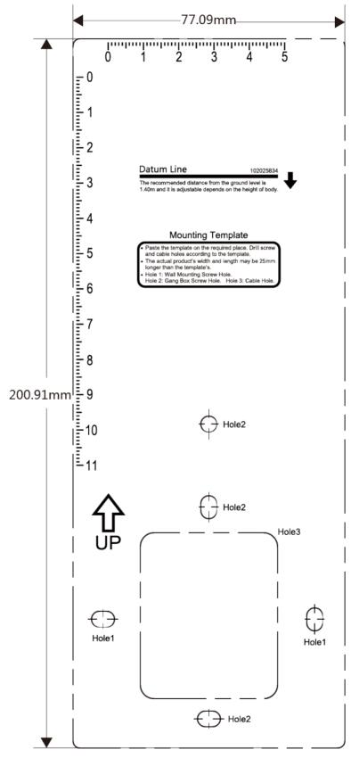
Figure 3-4 Mounting Template
