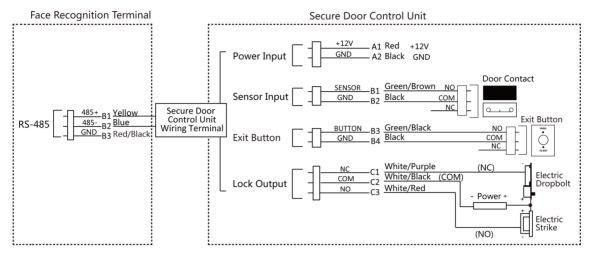
Figure 4-3 Secure Door Control Unit Wiring
