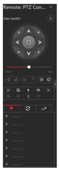
**Figure 14-9 PTZ Control Panel**
