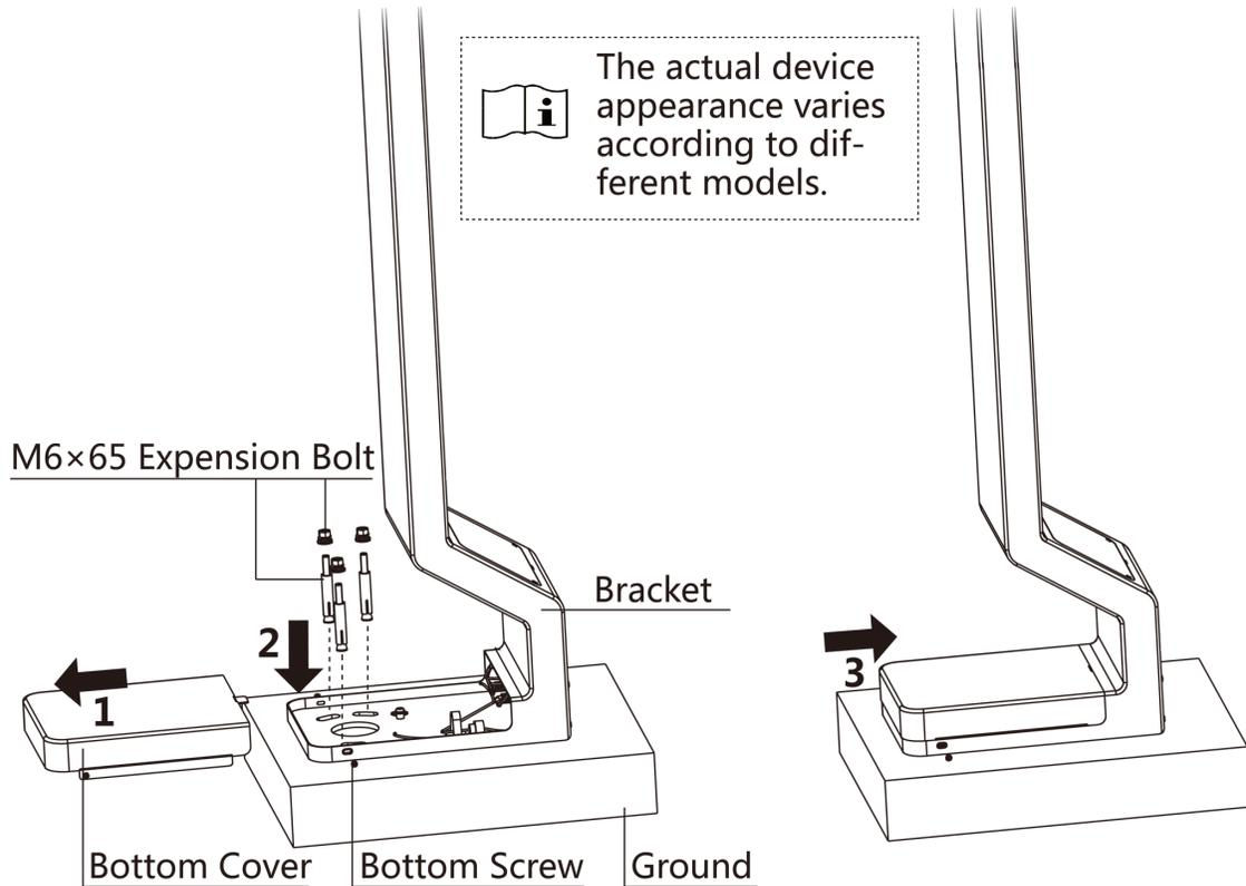
**Figure 3-1 Install Device**
