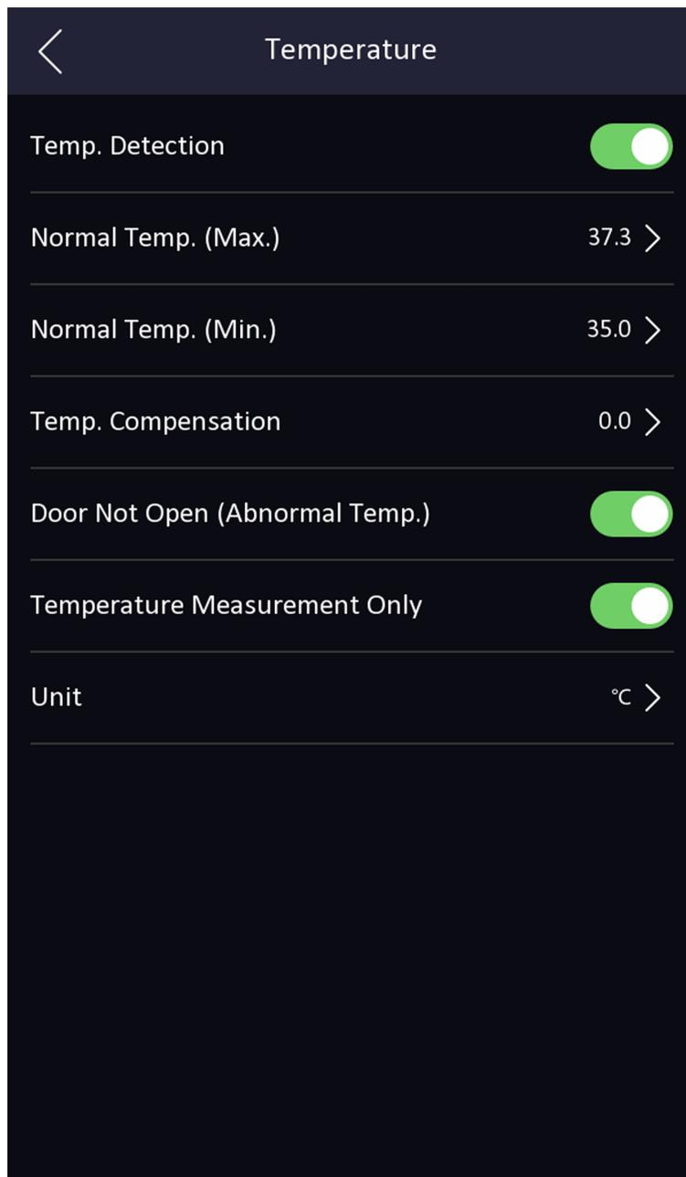
**Figure 7-9 Temperature Measurement Parameters**
