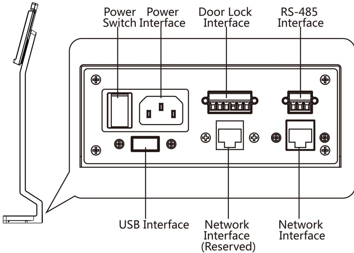
Figure 4-1 Wiring Interface
