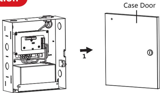
1. Open the case door with key and disassemble the case door.
