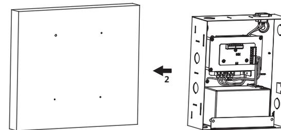
2. Secure the case body on the mounting area.
