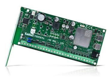
(e.g. to a security agency monitoring station), voice messaging, SMS control and audio verification (listening in to sounds from protected premises). It supports dual nano–SIM cards to ensure uninterrupted communication: if communication with the first operator's network fails, the second card is automatically selected.
