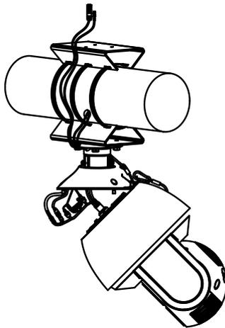
Figure 3-25 Fix the Speed Dome with Head Cover
