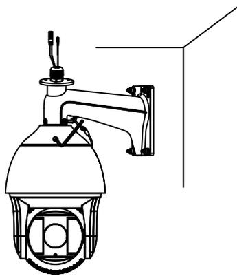
Figure 3-16 Fix the Speed Dome with Head Cover
