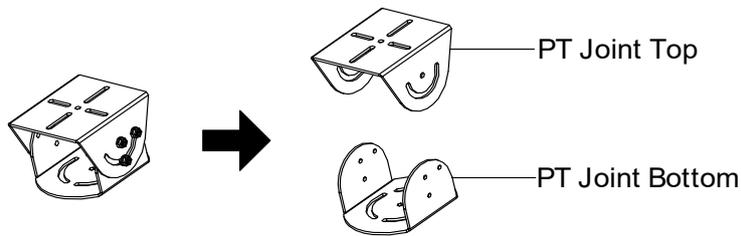
Figure 3-27 Disassemble the PT Joint
