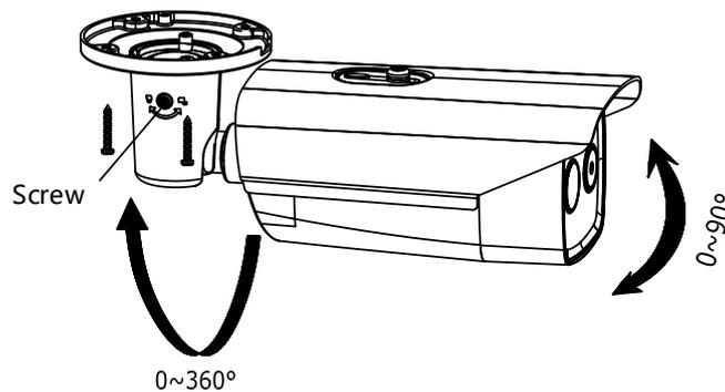
Figure 3-31 2-axis Adjustment
