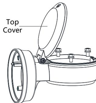
Figure 3-17 Open the Top Cover of Junction Box
