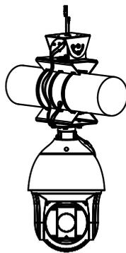
Figure 3-28 Bracket Installation
