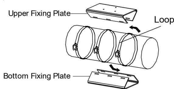
Figure 3-9 Install the Loop to the Pole
