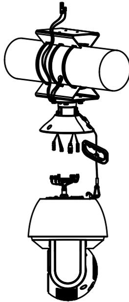
Figure 3-24 Hook the Safety Rope
