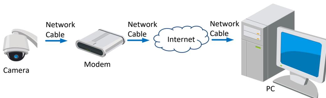
Figure 4-10 Accessing the Speed dome with Dynamic IP
