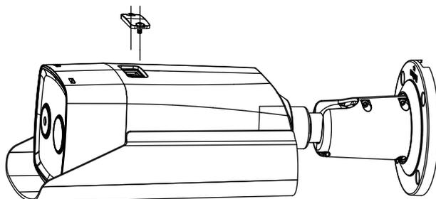
Figure 3-2 Open the Memory Card Slot
